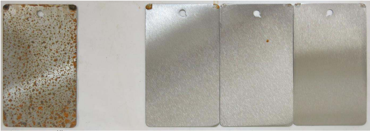
Figure 1: ASTM (1) D-1735 test results with Product A. The control panel is pictured on the far left.
