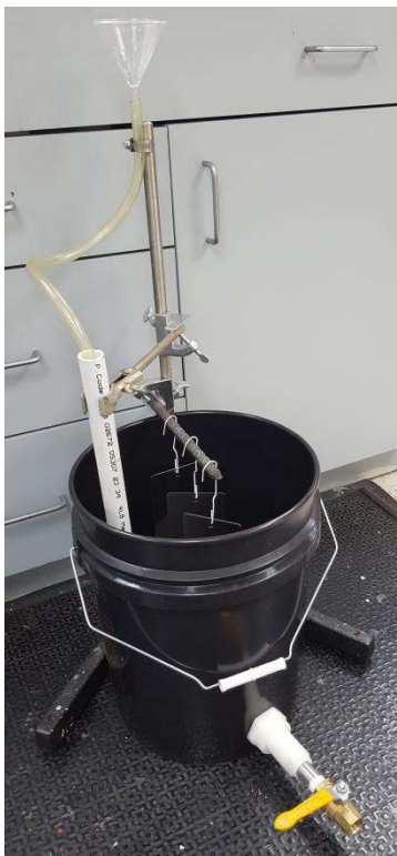
Figure 4: Total view of the float coating test vessel. Test panel holder, funnel and tubing for bottom-up filling of the vessel, and drain spout can be seen.
