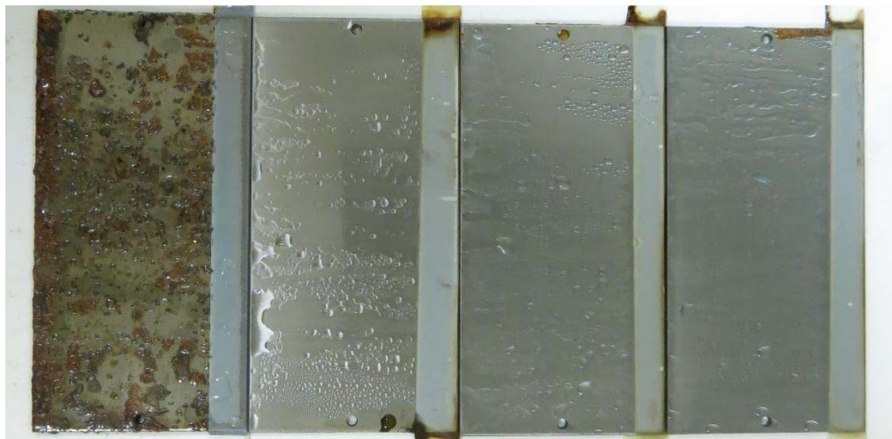
Figure 2: ASTM (1) D-1748 test results with Product A. The control panel is pictured on the far left.
