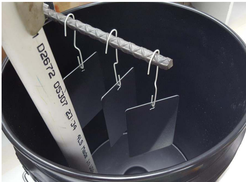
Figure 3: Image of the inside of the float coating test vessel. The vessel can accommodate several standard 4" x 12" test panels (3" x 5" test panels pictured above).
